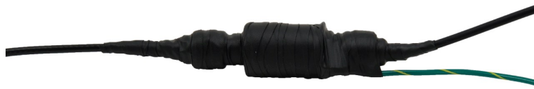
Figure 8-6. Properly weatherproofed antenna cable connection with surge protection
