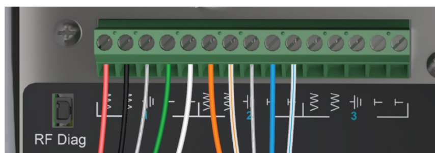
Figure 7-2. Typical vibrating-wire sensor wire colours and connections
